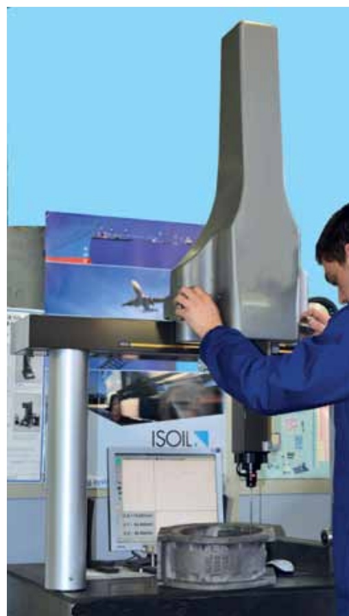
3D three-dimensional check of some components by a 3D machine.
