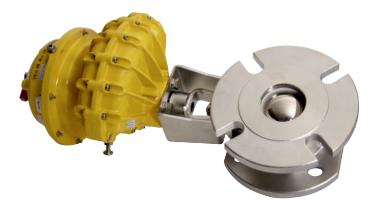
2" Pneumatically Operated Air Inlet Ball Valve - inlet flange drilled 4 x 18mm holes on a 125mm PCD; outlet flange 4 x 18mm open slots on a 120.7mm minimum PCD to suit 2" ASA 150/DIN50 PN40. Valve manufactured in 316 stainless steel with PTFE seals. Fitted with Kinetrol pneumatic actuator with spring return and  $\frac{1}{4}$ " BSP air inlet.
