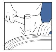
Knock the seal firmly into place with a plastic or wooden mallet, all round the manlid
