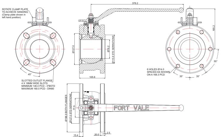
3" Blacko Ball Valve Assembly - inlet flange drilled 6 x 14mm holes on a 168mm PCD. Slotted 4 hole outlet flange. Left hand operated. Contact parts manufactured in 316 stainless steel with PTFE seals.
