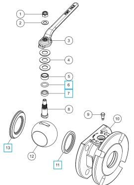
2" Full Bore Blacko Ball Valve - inlet flange drilled 4 x 18mm holes on a 125mm PCD (DIN50 PN16); outlet flange with 4 x 18mm open slots on a 120.7mm minimum diameter to suit 2" ASA150 and DIN50 PN40. Left hand operated with TIR facility to handle. Contact parts manufactured in 316 stainless steel with PTFE seals.
