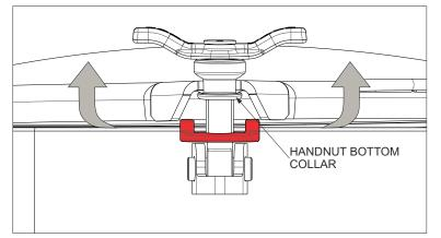
When intentionally unscrewed, the bottom collar on the handnut forces the lid to open slightly, even if the gasket is sticking to the neckring. This allows any residual pressure inside the tank to vent, making it safe for the operator to open the lid.
