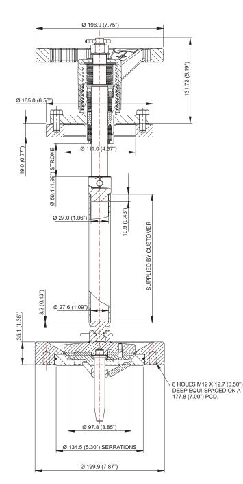
4" Screwdown Valve - comprising: top tank weld-in pad, stud kit and PTFE gasket; spring-loaded top operator; 4" poppet assembly with PTFE seal disc; 4" NB bottom tank weld-in pad with replaceable seat area. Contact parts manufactured in 316 stainless steel. NOTE : 1" Sched. 10 tube not supplied.
