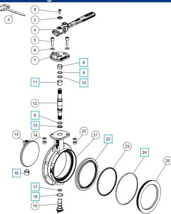
100mm Clamped Butterfly Valve - drilled TW100. Designed to clamp between two TW100 flanges with the bolts passing through the valve body holes. Left hand operated lockable handle with T.I.R. Contact parts manufactured in 316 stainless steel with Flextyt main seal.
