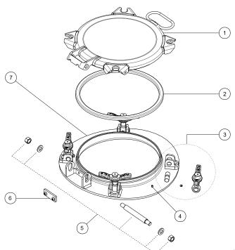
300mm Ultra Low Profile Inspection Hatch Assembly -4 point fastening double skin cover. 8mm thick pressed neck/compensating ring profiled to suit tank radius range from 750 to 1220mm. Contact parts manufactured in 316 stainless steel. Stainless steel swingbolts with naval brass handnuts. Seal supplied separately.
