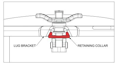
In this position, the safebolt retains the manlid closed, as does a standard swingbolt. In the event of the handnut working loose, the retaining collar (shown in red) will prevent the swingbolt from pivoting away from the lug bracket, thus preventing the manlid cover from opening suddenly due to a build-up of pressure inside the tank.
