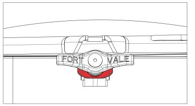
Only when the safebolt has been fully unscrewed will the retaining collar be clear of the manlid lug bracket, allowing the bolt to pivot and the manlid to open fully.
