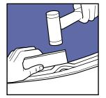
If a kink occurs, use a small piece of clean plastic or spare seal material and the mallet to work the seal back into the groove
