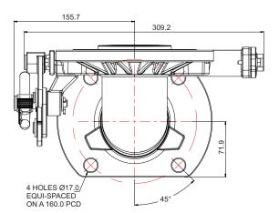
3" 90° Cleanflow Footvalve - inlet flange drilled 8 x 14mm holes equi-spaced on a 178mm PCD; outlet flange drilled 4 x 17mm holes equi-spaced on a 160mm PCD with flats milled top and bottom. Footvalve body with 'Superseat' (alloy 625) seating area. All other contact parts manufactured in 316 stainless steel with Fortyt O ring to main poppet as standard.
