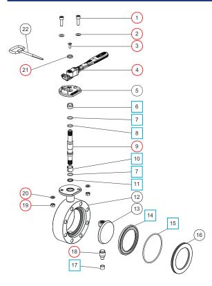
80mm Clamped Butterfly Valve - drilled TW 80. Designed to clamp between two TW80 flanges with the bolts passing through the valve body holes. Left hand operated lockable handle with T.I.R. Contact parts manufactured in 316 stainless steel with PTFE seal.
