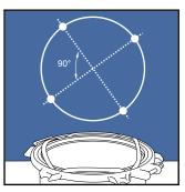
Push the seal into the manlid groove at four points, 90° to each other
