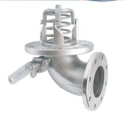
3" 90° Tankstream Footvalve - 3" to 3" 90° footvalve assembly. Inlet flange drilled  $12 \times 14$ mm holes on a 6.25" PCD. 6 inlet holes are plugged with a plastic plug. Outlet flange drilled 8 x 10.5mm holes on a 124mm PCD. Contact parts manufactured in 316 stainless steel with Fortyt or Viton O ring.
