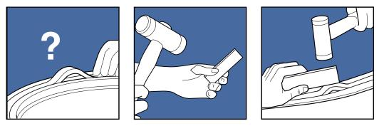
If a kink occurs, use a small piece of clean plastic or spare rubber seal material and the mallet to work the seal back into the groove.
