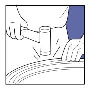
Knock the seal firmly into place with a plastic or wooden mallet, all around the manlid
