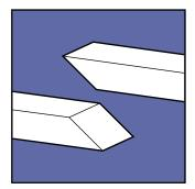
Take the braided seal and place it over the manlid groove to measure the length required. Cut the seal with a mitre joint. PTFE tape may be applied to reinforce the mitre joint. (Adhesive not recommended)
