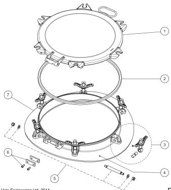
500mm Pendle Manlid Assembly - 6 point double skin manlid cover, hinged to open to 135°. Deep pressed neck/compensating ring, 51mm in height, profiled to suit a tank radius of between 850mm and 1220mm. To suit a MAWP of 3 Bar. Contact parts manufactured in 316 stainless steel with stainless steel swingbolt assemblies. Seal supplied separately.
