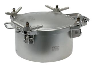
500mm Rail Manlid Assembly - 4 point fastening. To suit a MAWP of 3 Bar. 10mm thick x 250mm deep neckring. Contact parts manufactured in 316 stainless steel. Seal supplied separately.
