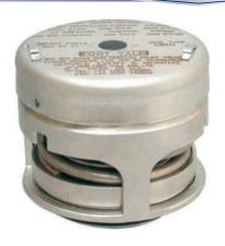
M90 x 2mm 65mm NB MK3 Super Maxi Relief Valve - M90 x 2mm threaded connection with 65mm to 80mm tapered nominal bore. Suitable for a pressure range of between 2 - 75 PSI (0.14 - 5.17 bar) and a vacuum range of between 0 - 24" Hg (0 - 0.81 bar). Contact parts manufactured in Alloy C276 with Halar coated pressure springs and Alloy C276 vacuum springs. Fitted with Fortyt seals as standard. Complete with rubber/PTFE tank seal.
