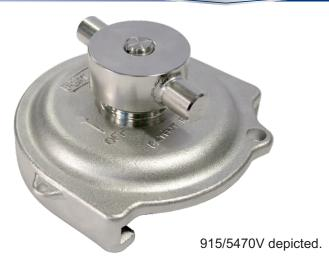
The pressure-tight cap can be used as a secondary or tertiary closure and is designed to safely release any build-up of pressure from the tank unit. It is firesafe designed and seals metal-to-metal when installed on the tank unit. In addition, the sealing plate O ring enables a gas-tight and liquid-tight seal. (\*\*exception applies, see Specification)
