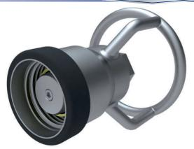
50mm Rail Locomotive Fuel Delivery Coupler - 1½" BSP inlet, 50mm outlet. Inner housing manufactured in brass and aluminium for smooth operation and to prevent galling. The design of the poppet ports facilitates optimum flow rate of fuel. Robust outer housing manufactured in stainless steel for improved corrosion resistance and longevity. Fitted with Viton main seal.
