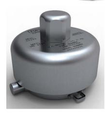
3" BSP Female Vacuum Vent Valve - suitable for a vacuum range of between 0.5"Hg to 6.2"Hg (0.02 Bar to 0.21 Bar). Manufactured in 316 stainless steel fitted with Fortyt seal. Fitted with weatherproof cowl and gauze ring.
