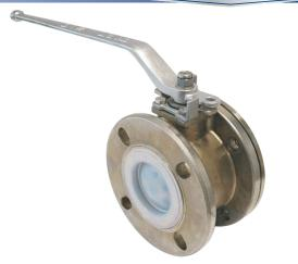
PFA Lined 80mm Full Bore Ball Valve - inlet flange drilled 4 x 18mm holes on a 160mm PCD; outlet flange drilled 4 x 18mm slots equi-spaced on a 146 to 160mm PCD. (3" BSTD to DIN80) Left hand operated with TIR to handle. Valve manufactured in stainless steel with PTFE main seal. All parts in contact with the cargo lined with PFA.
