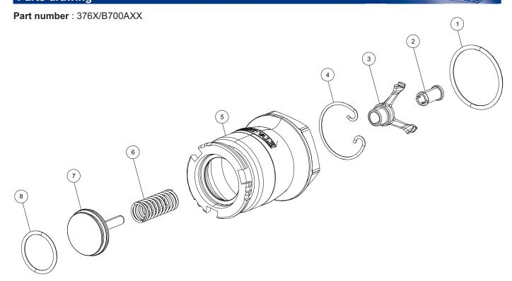
Description Part number Item PTFE O ring ORB832P0 2 Guide bush 376/0702/2 Spider 376/B702 3 4 Snap ring 5120-081 70mm "Drytyt" coupler body 5 376/B701AXX \*See Note 5104-800 6 Poppet spring 376/B703 Poppet assembly Poppet O ring \*See Table 1 5005-XXXX 8
