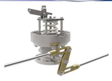
5" 180° Rail Footvalve - with dual handle assembly. Inlet flange drilled 8 x 18mm holes on a 210mm PCD. Outlet flange drilled 8 x 18mm holes on a 200mm PCD. Contact parts manufactured in 316 stainless steel. Fitted with PTFE/Elastomer main seal. Non contact parts manufactured in 304 stainless steel / mild steel.
