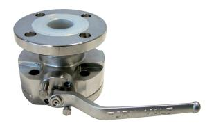
PFA Lined 50mm Full Bore Flanged Ball Valve - inlet flange drilled 4 x 18mm holes on a 126mm PCD; outlet flange drilled 4 x 18mm slots on a 120.7mm to 127mm PCD. Valve manufactured in stainless steel with PTFE main seal. All parts in contact with the cargo lined with PFA.
