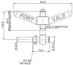
M24 Forged Swingbolt Assembly - designed and manufactured in accordance with BS EN12561-6. To suit rail tank manlid assembly. Manufactured in 316 and 304 stainless steel.
