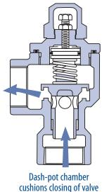
In operation, Blackmer valves provide exceptionally close pressure control, even under widely varying bypass flow conditions. The performance curve in Figure 2 shows how a Blackmer valve maintains a virtually constant pressure of 100 psi (6.89 bar) even as the volume being bypassed rises
