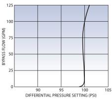
FIGURE 2. Bypass volume/pressure curve BV1.5
