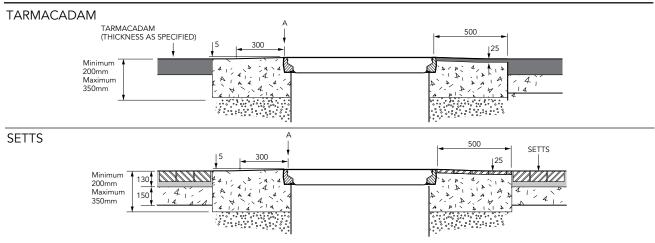
1.2m square base chamber with a sealed corbel, adjustable skirt, non-structural internal lid and round 900mm flat sealed cover. 1.2m2 tank flange detail
