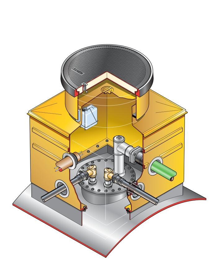
1.2m square base chamber with a sealed corbel, adjustable skirt, non-structural internal lid and round 900mm flat sealed cover. 1.2m2 tank flange detail
