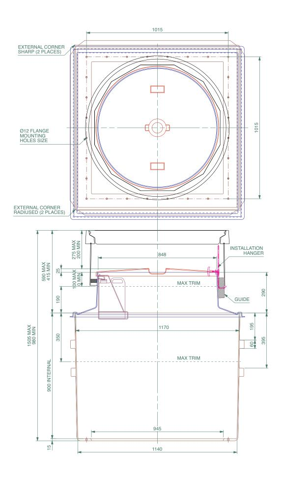
1.2m square base chamber with a sealed corbel, adjustable skirt, non-structural internal lid and round 900mm flat sealed cover. 1.2m2 tank flange detail
