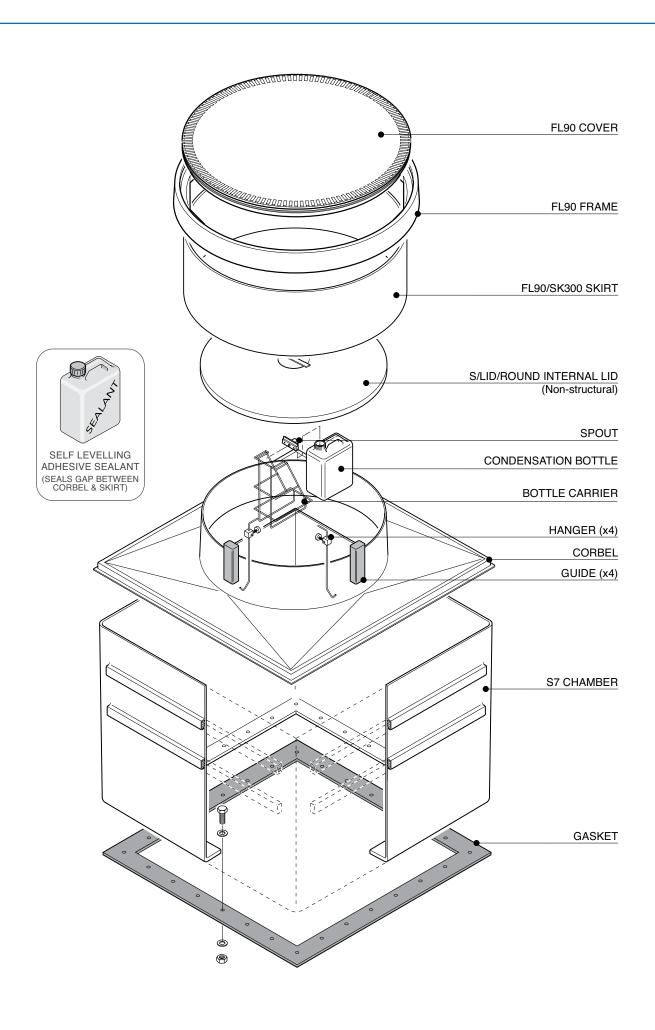
1.2m square base chamber with a sealed corbel, adjustable skirt, non-structural internal lid and round 900mm flat sealed cover. 1.2m2 tank flange detail
