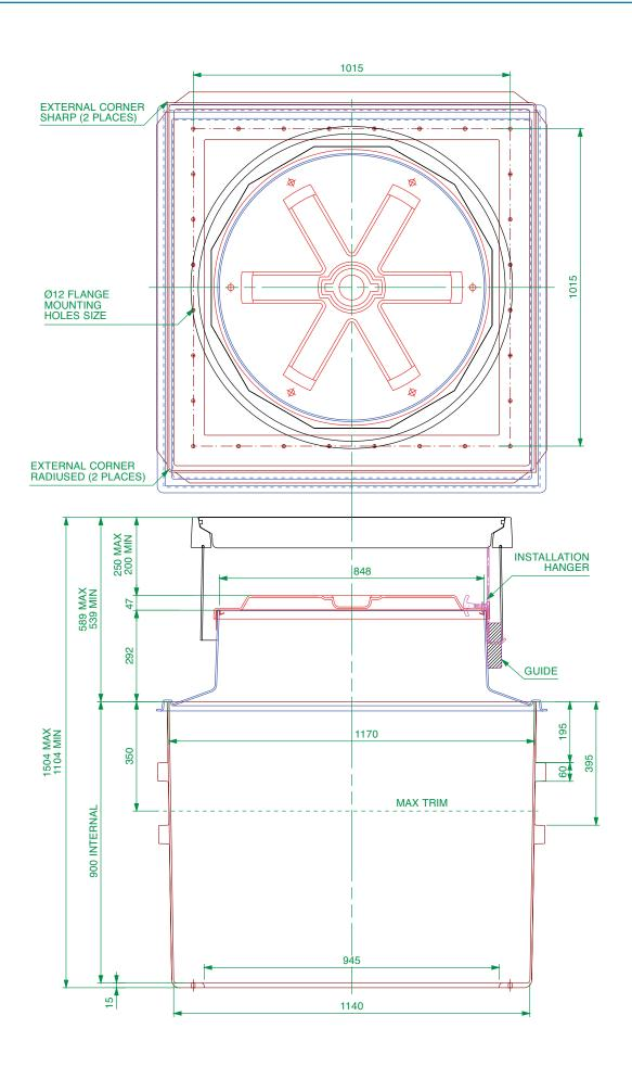
1.2m square base chamber with a sealed corbel, adjustable skirt, internal watertight platform and round 900mm flat sealed cover. 1.2m2 tank flange detail
