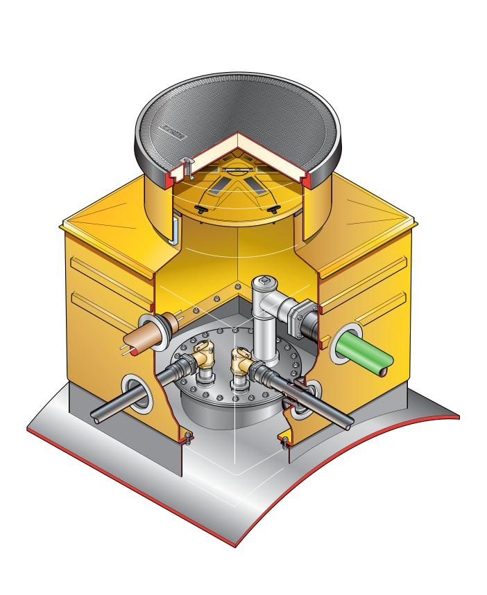
1.2m square base chamber with a sealed corbel, adjustable skirt, internal watertight platform and round 900mm flat sealed cover. 1.2m2 tank flange detail
