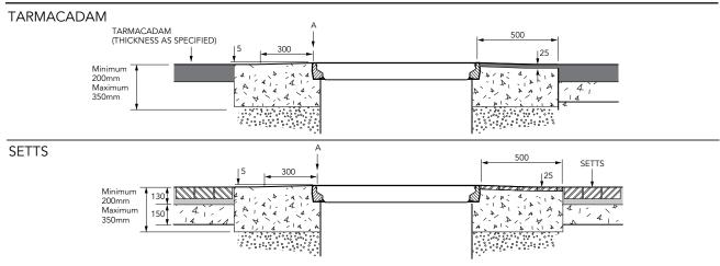
1.2m square base chamber with a sealed corbel, adjustable skirt, internal watertight platform and round 900mm flat sealed cover. 1.2m2 tank flange detail
