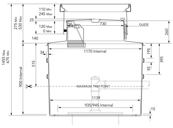
1.2m square base chamber with a sealed corbel, adjustable skirt and square flat sealed 760mm cover. 1.2m tank flange detail.
