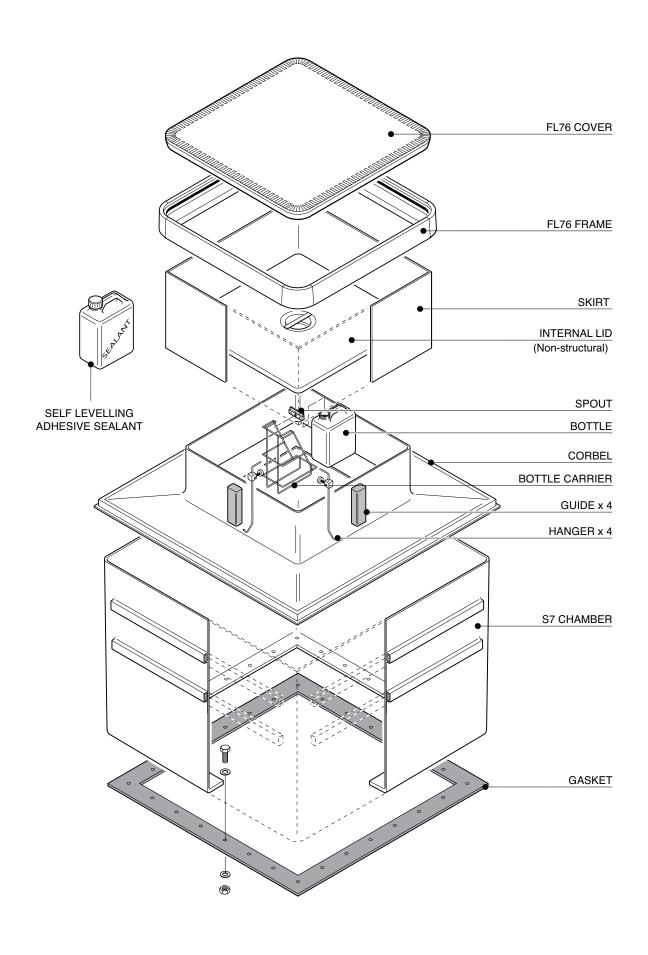
1.2m square base chamber with a sealed corbel, adjustable skirt and square flat sealed 760mm cover. 1.2m tank flange detail.
