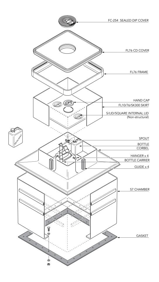
1.2m square base chamber with a sealed corbel, adjustable skirt, non-structural internal lid and square 760mm flat sealed cover with a central dip cover 1.2m2 tank flange detail
