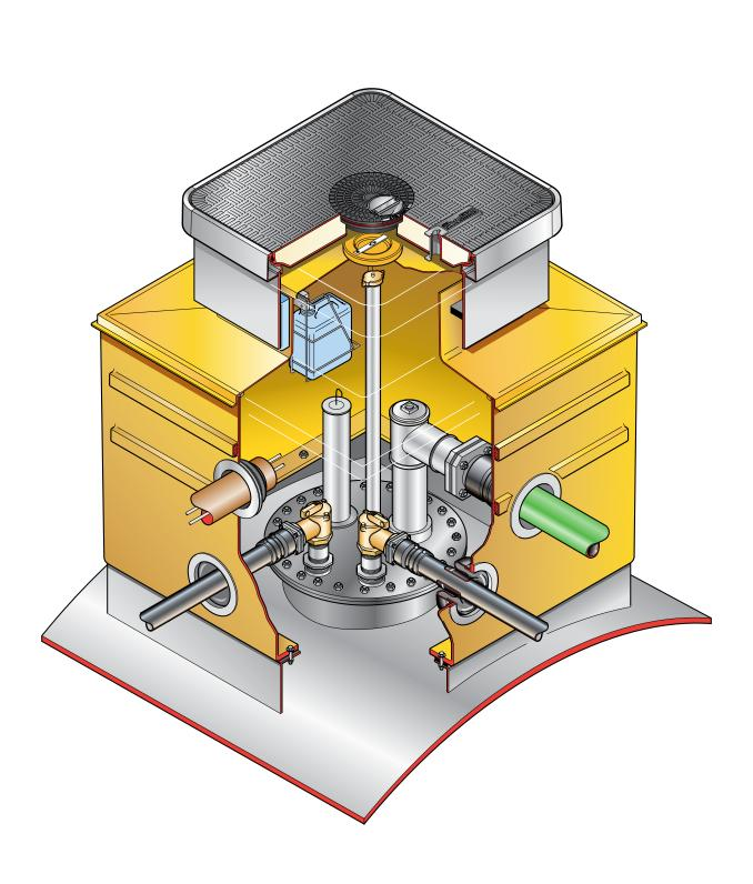
1.2m square base chamber with a sealed corbel, adjustable skirt, non-structural internal lid and square 760mm flat sealed cover with a central dip cover 1.2m2 tank flange detail
