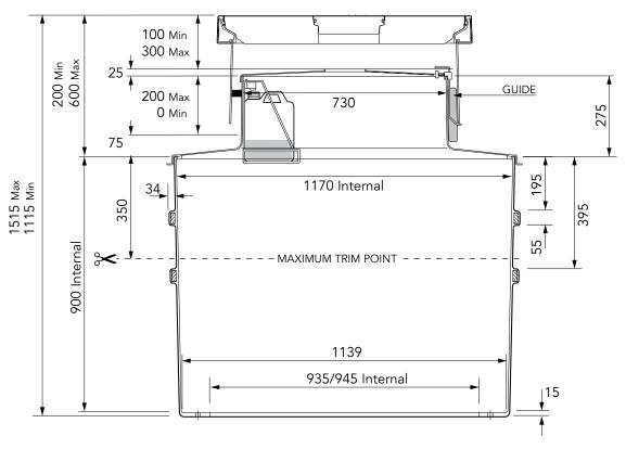
1.2m square base chamber with a sealed corbel, adjustable skirt, non-structural internal lid and square 760mm flat sealed cover with a central dip cover 1.2m2 tank flange detail
