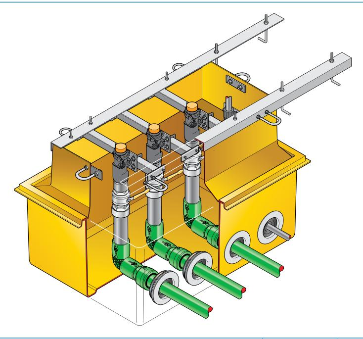
1100mm x 800mm GRP solid base sump and corbel to fit Gilbarco SK700 1/2 dispenser model. Includes dispenser support rails, shear valve rail and all fixings. KPS pipework and Fibrelite entry boots.
