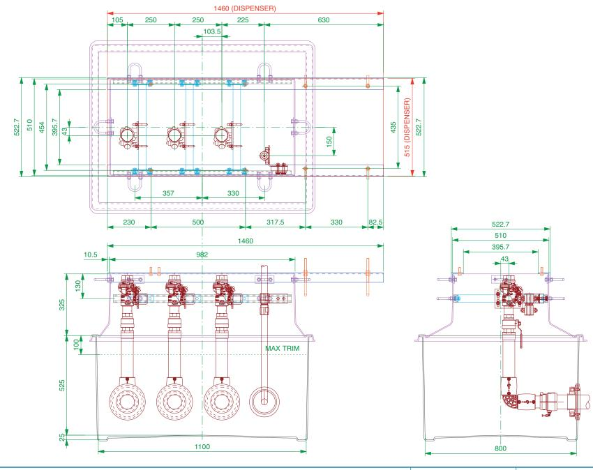
1100mm x 800mm GRP solid base sump and corbel to fit Gilbarco SK700 1/2 dispenser model. Includes dispenser support rails, shear valve rail and all fixings. KPS pipework and Fibrelite entry boots.
