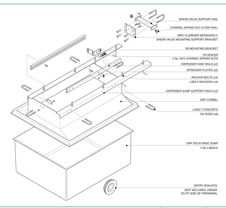
1100mm x 800mm GRP solid base sump and corbel to fit Gilbarco SK700 1/2 dispenser model. Includes dispenser support rails, shear valve rail and all fixings. KPS pipework and Fibrelite entry boots.
